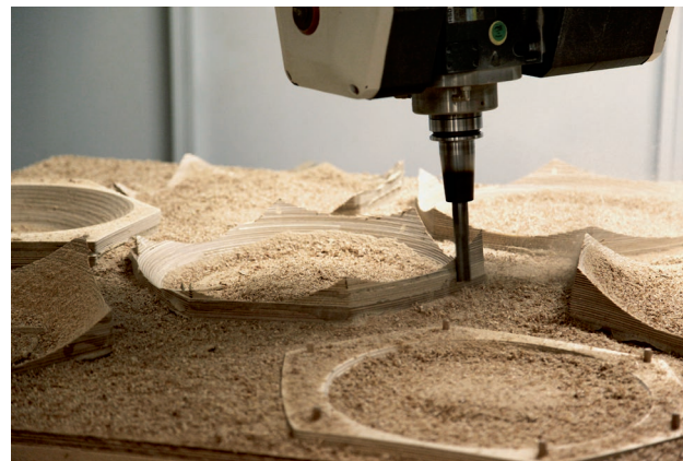
Fig. 8: Swarf milling the voussoir edges.
